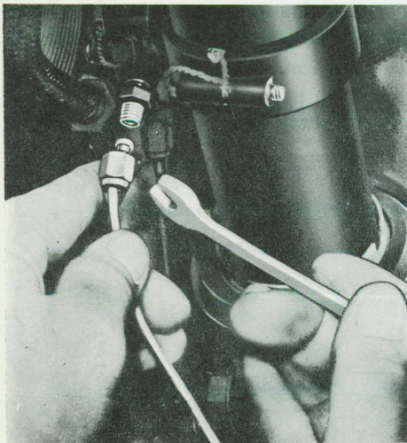
Figure 6-27 Primer Line at Distributor
